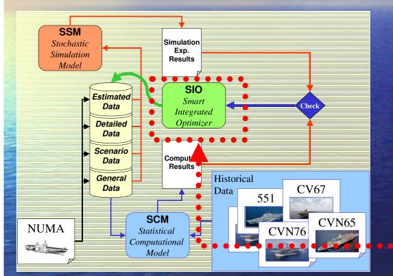
SIO proceeded to an automates optimization devoted to obtain a best fit setting of detailed parameters based on the comparison between SCM and SSM
