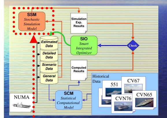
The SSM is a stochastic simulator that reproduce Carrier operation during whole life cycle considering different expected scenario; the results obtained by this model on traditional operative scenario can be compared with the SCM
